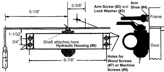
Refer to the Assembly Drawing on page 5. **Note:** Diagram above is showing right hand opening; left hand opening would layout in opposite direction.
